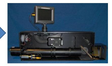
• Then remove the two screws that hold the fan housing to remove it also. The fan is not completely non-magnetic, so place it above the Eyetracker.
