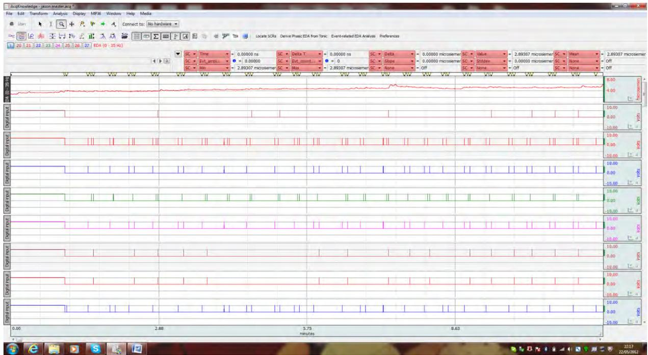
The trigger events have now been integrated into the main EDA signal and are signified in the event bar as the light-bulbs (i.e., stimulus delivery events). Once this step has been completed, the trigger channels can be hidden so that the observer can get a better look at the EDA signal. Simply hold down the Alt key while clicking on the channel number button - you can toggle the visibility of any given channel (hide or make visible).
