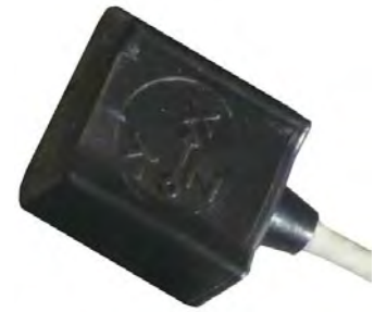
Tri-axial accelerometer uses 3 channel inputs
