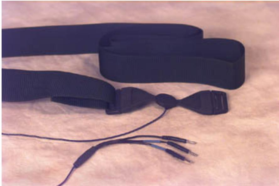
To attach the nylon belt to the respiration transducer, thread the nylon strap through the corresponding slots on the bow tie so the strap clamps into place when tightened. The TSD101B is placed around the area of maximal expansion when the subject breathes, generally about 5 cm below the armpits and should be fitted so that it is snug.
