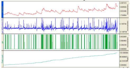
4. To measure the number of changes in a given period (e.g., following an event or at user-defined intervals), use the "delta" measurement on the Count peak waveform.
